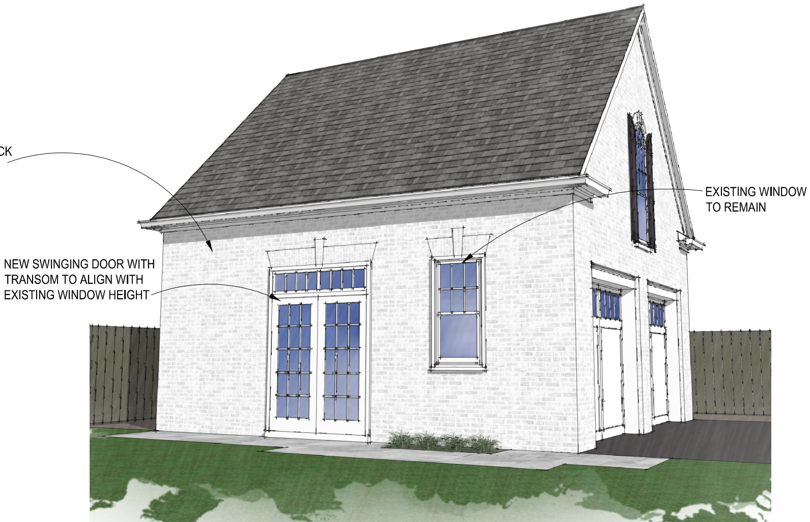
2 PROPOSED LEFT SIDE ELEVATION THIS ELEVATION NOT VISIBLE FROM STREET Scale: N.T.S.
