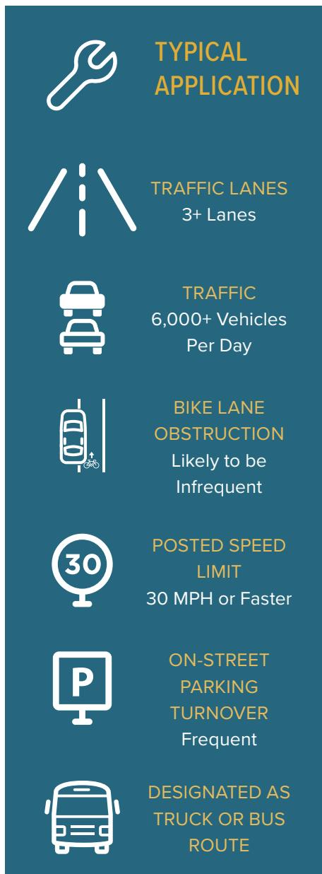
Figure 8-3: Typical application of separated bikeways
