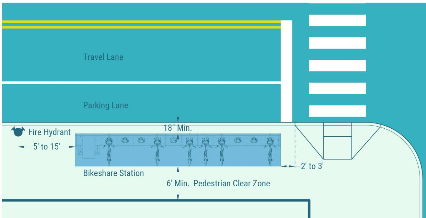
Figure 4-8. Example of bikeshare station clearances on the sidewalk (Graphic modified from NACTO Bike Share Station Siting Guide, <https://nacto.org/publication/bike-share-station-siting-guide/>)
