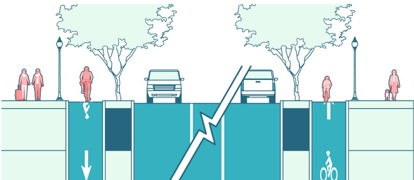
Figure 8-10: One-way Separated Bike Lane, Tree Separated, Permanent Condition: **Downtown Street, Town Center Street, Industrial Street**
