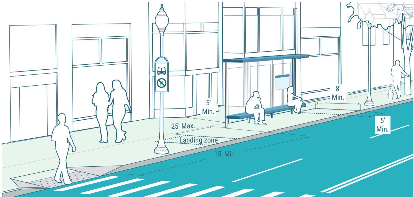
Figure 4-19. Illustration of bus shelter clearances
