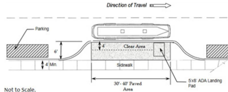
Figure 6-24. Bus Bulb design
