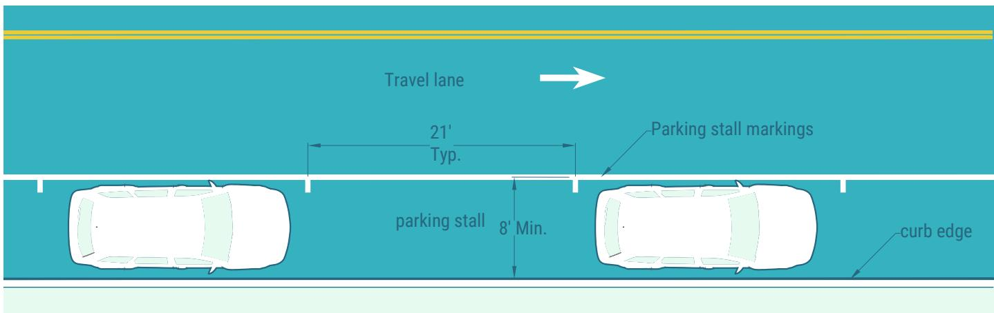
Figure 5-5. Illustration of a typical on-street parallel parking space with dimensions
