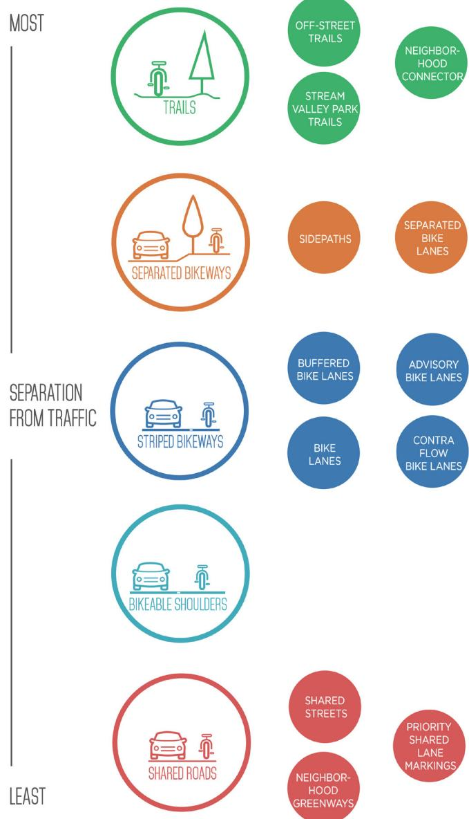
Figure 8-1: Montgomery County bikeway facility types
