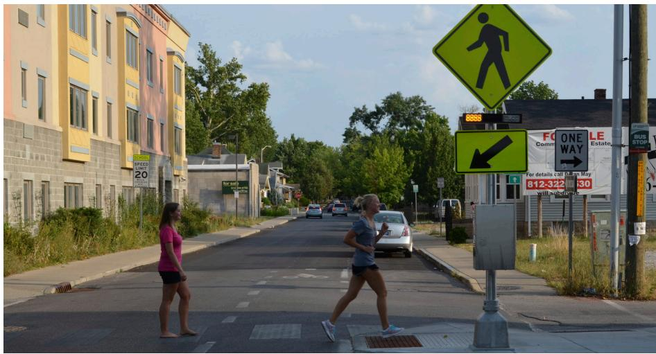
Figure 6-31. A Rectangular Rapid Flashing Beacon (RRFB)
