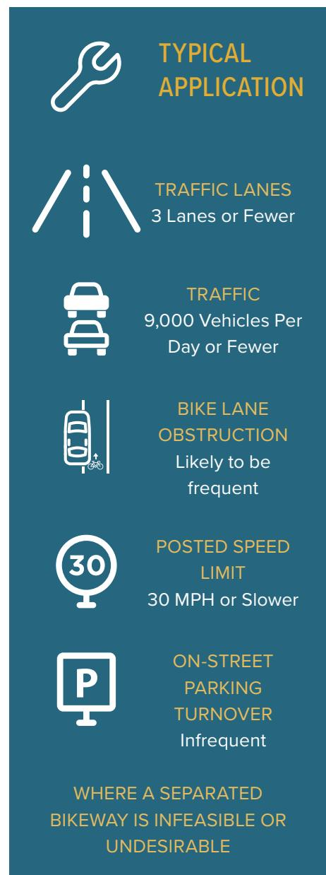
Figure 8-14: Typical application of striped bikeways
