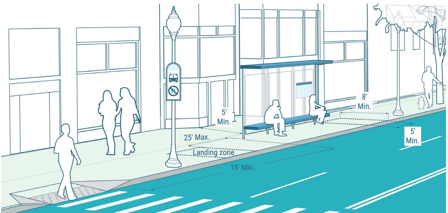
Figure 4-19. Illustration of bus shelter clearances
