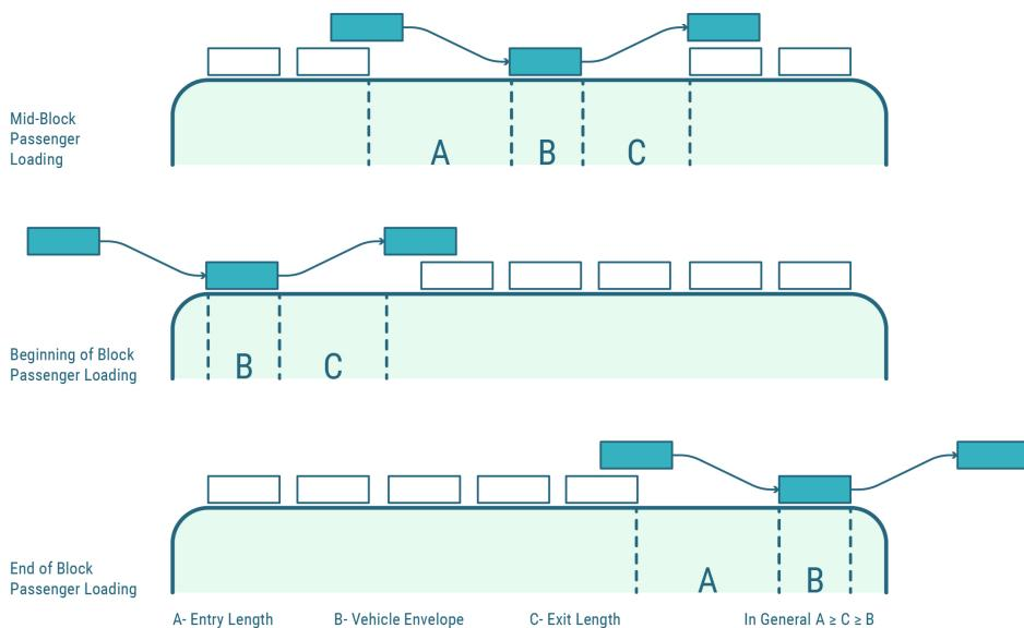
Figure 5-12. Ride hailing pickup/drop-off area diagrams (Graphic content from: ITE Curbside Management Practitioners Guide)
