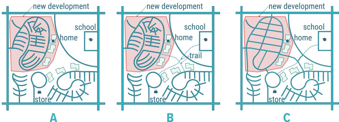
Figure 5-19. Examples of network connectivity and design
