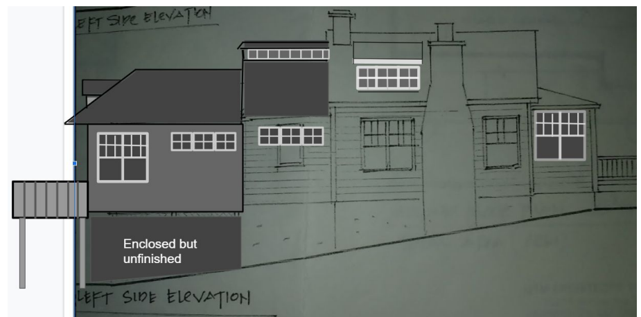
Side elevation: Shed Dormer window set dimensions 6 x 2 ft. 3 windows each 2x2 ft
