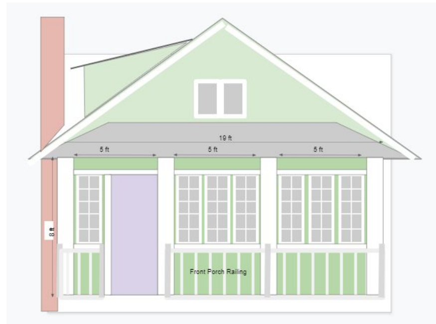
Side elevation: Shed Dormer window set dimensions 6 x 2 ft. 3 windows each 2x2 ft
