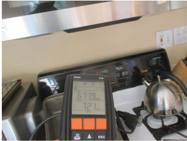
High CO reading from oven
