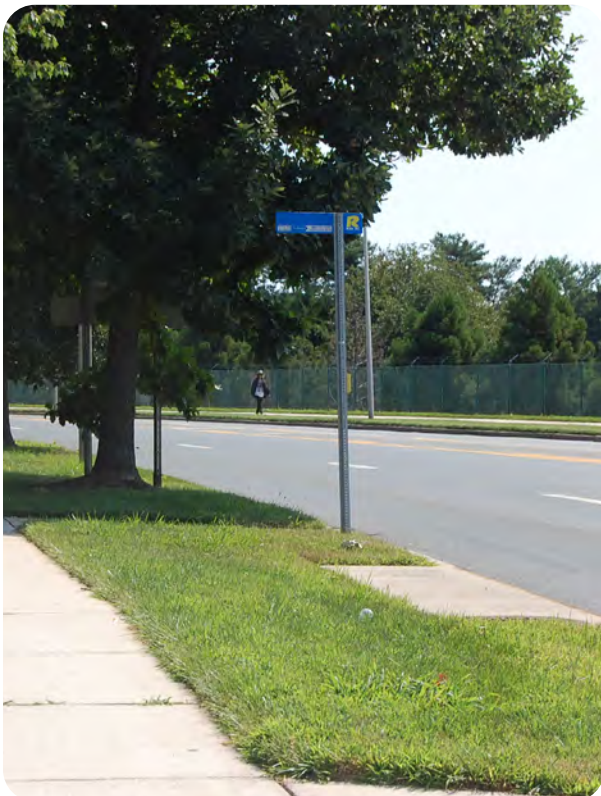
Buffers between the sidewalk and the road, as pictured here on Connecticut Avenue, should be at least five feet wide. Trees planted in the buffer provide additional protection for pedestrians and discourage speeding.
