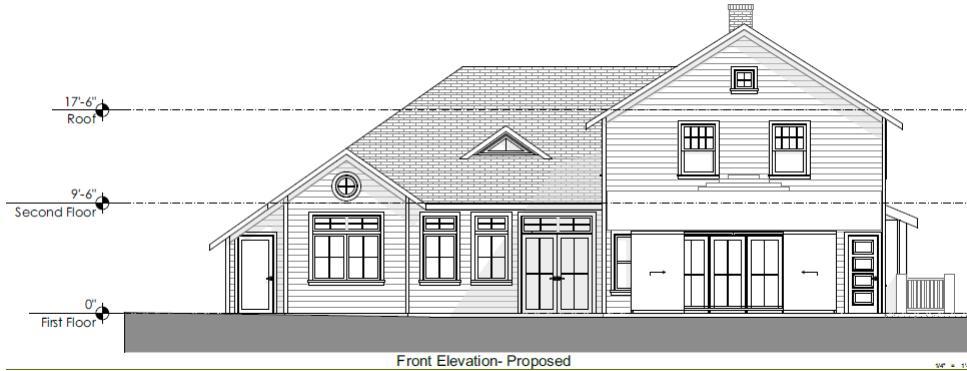
**Fig. 3: Current proposed front elevation, showing original garage doors to remain.**
