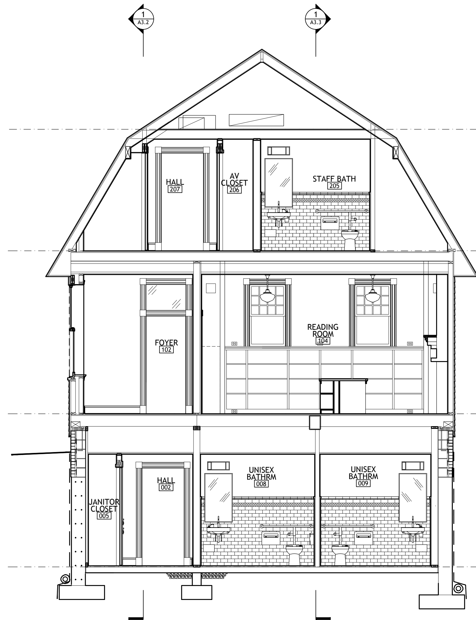
1 A3.4 BUILDING SECTION SCALE: 1/4" = 1'-0"
