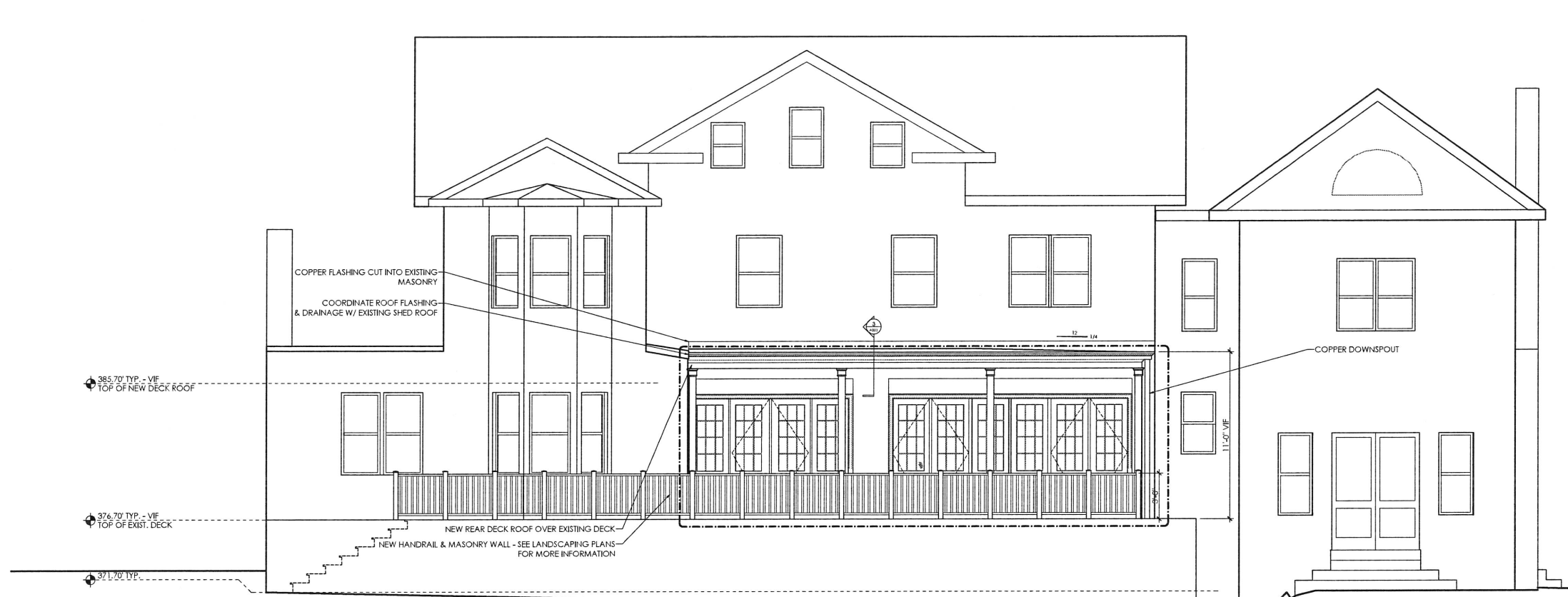
① REAR DECK ELEVATION SCALE: 1/4"=1'-0"
