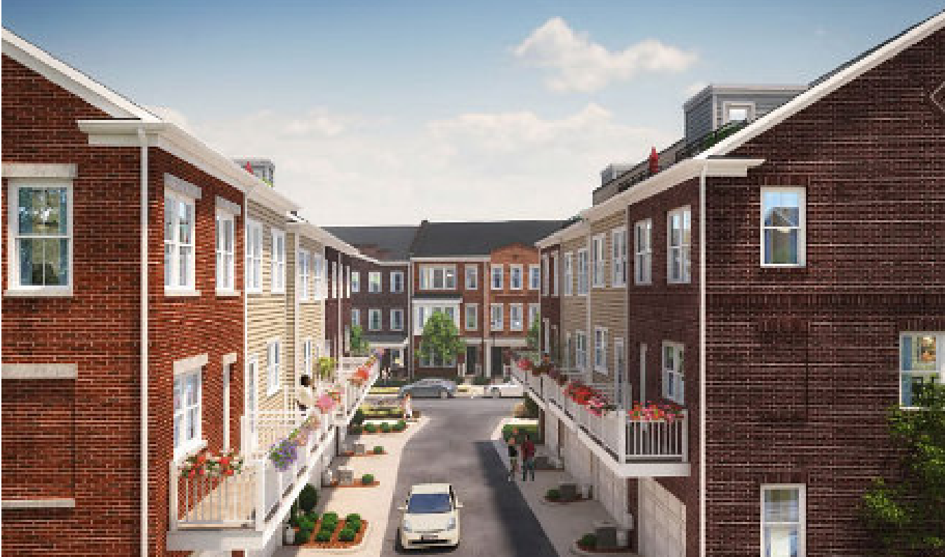
Figure 3.15: Alleyways, flanked by less than three-story townhouses, may be used to provide FDA if appropriately dimensioned
