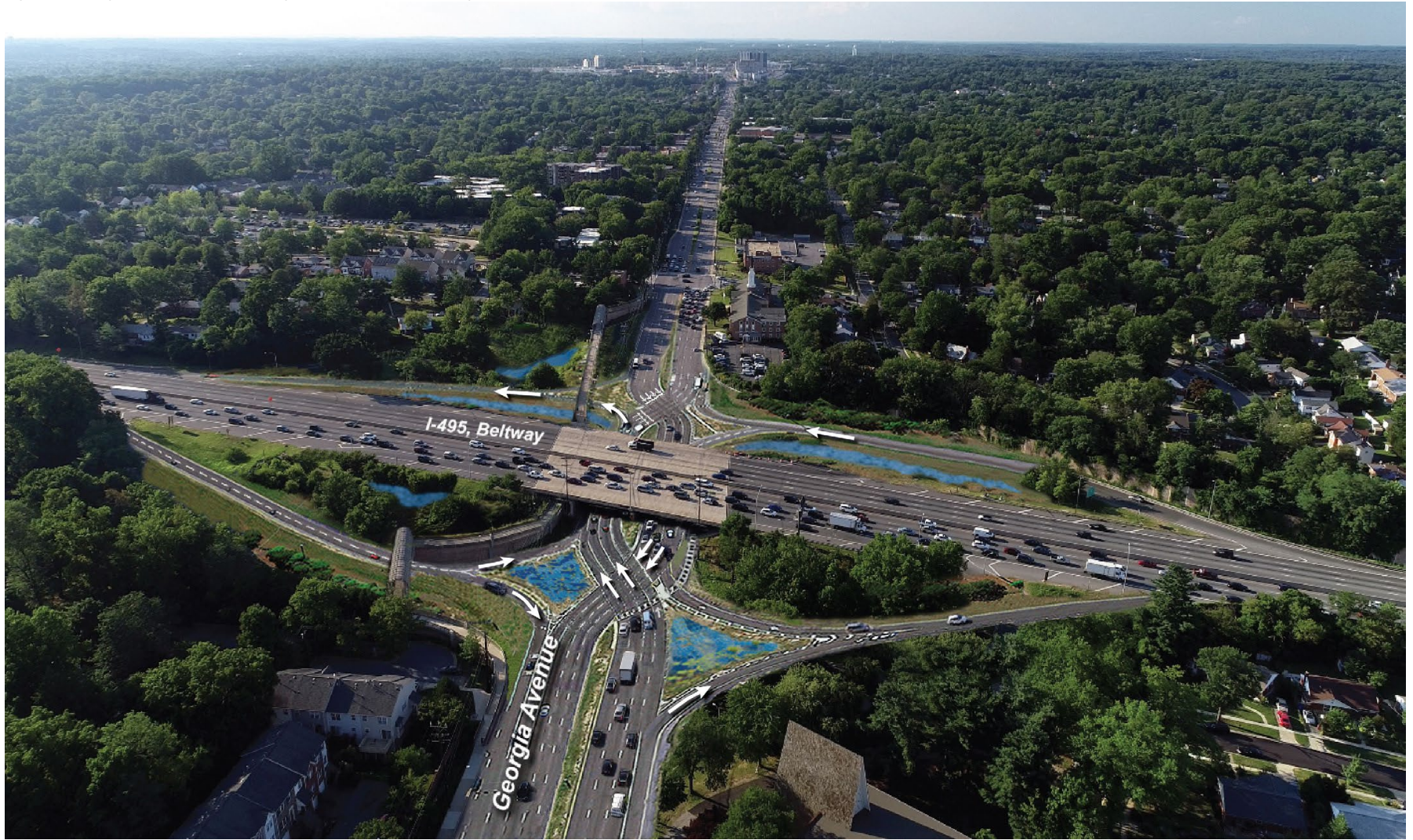
Figure 7: Design Alternative 2 – Divergent Diamond Interchange
