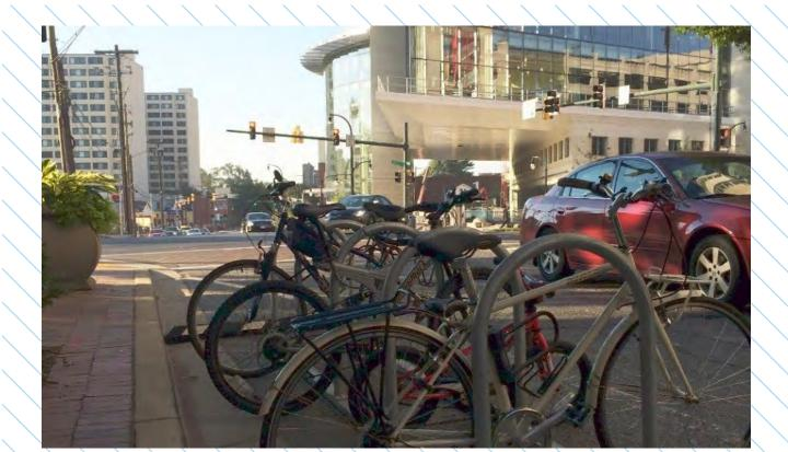
Where sidewalk space is limited, bike corrals, such as this temporary installation in Downtown Silver Spring, can expand the overall parking supply by converting one automobile parking space to between 8 and 12 bicycle parking spaces
