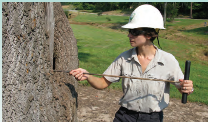
Probing may provide the risk assessor an approximation of the extent of decay.
