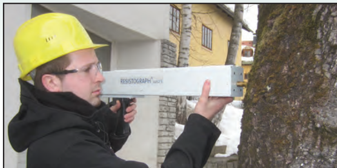
An inspector, with the proper training, can distinguish solid wood from decaying wood, with the use of a resistance-recording drill.
