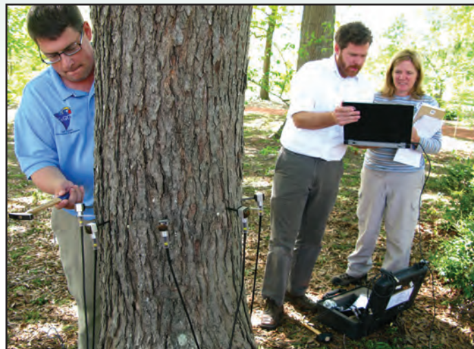
Sonic tomography instruments use measurements between many points to create a two- or three-dimensional picture (tomogram).
