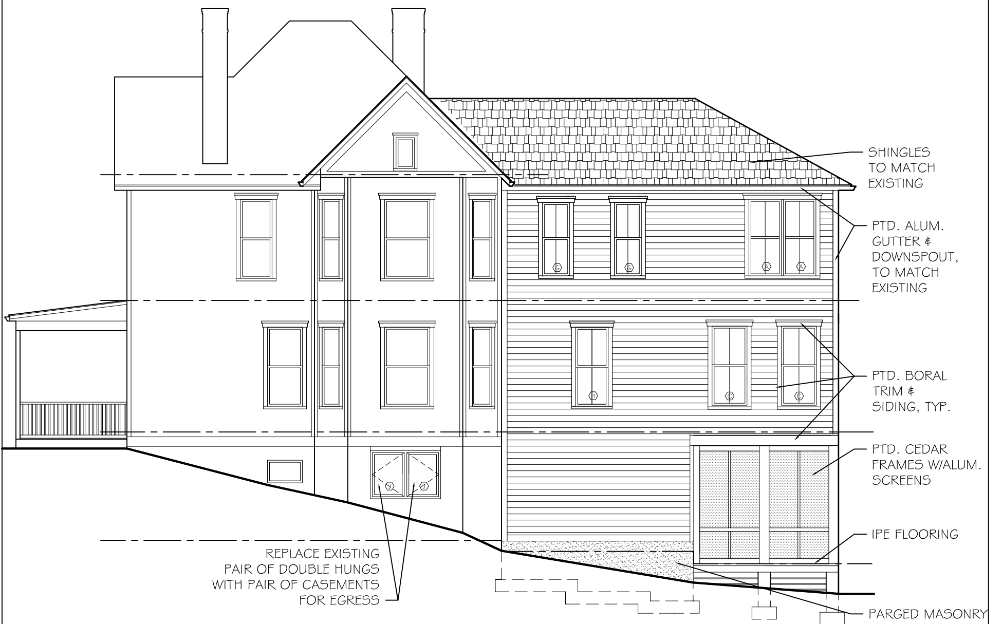
B 7 SOUTH ELEVATION - PROPOSED 1/8" = 1'-0"
