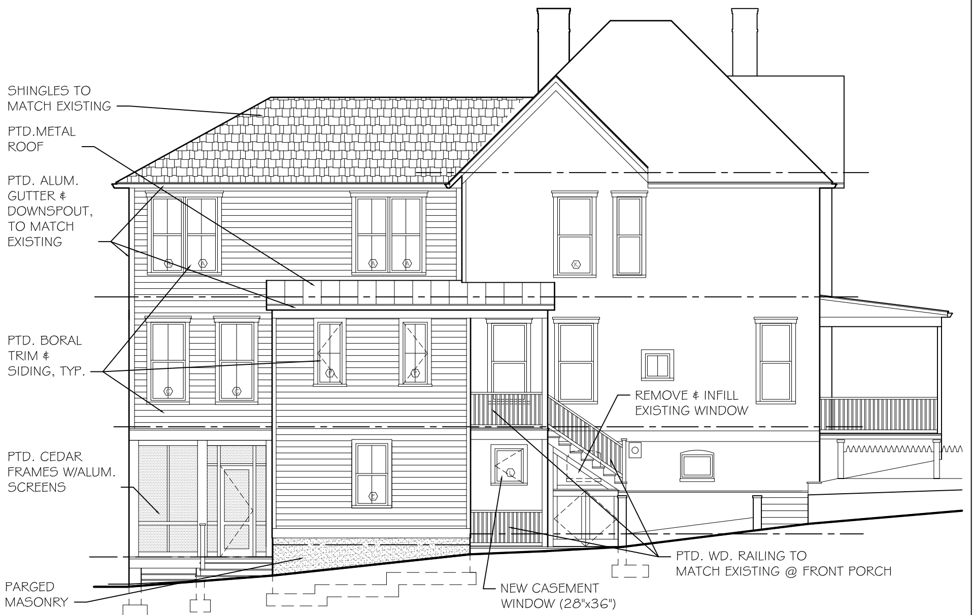
B 5 NORTH ELEVATION - PROPOSED 1/8" = 1'-0"
