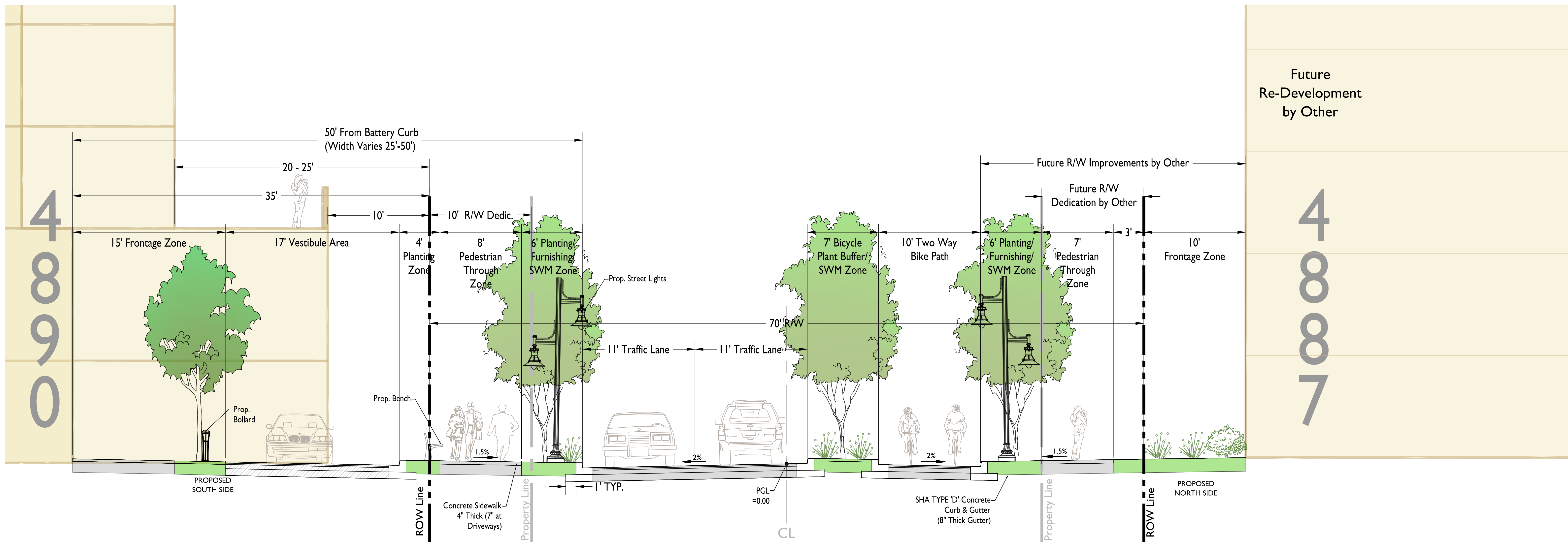
4890/4900 (TOWER I) PROPOSED BATTERY LANE ROAD SECTION
