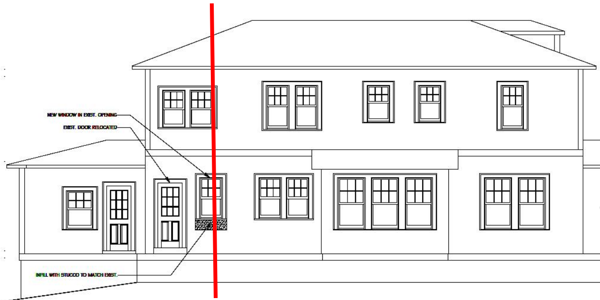
Fig. 8: Transition from the eaves of the historic hipped roof to the shed roof on the addition, as indicated by the red line.
