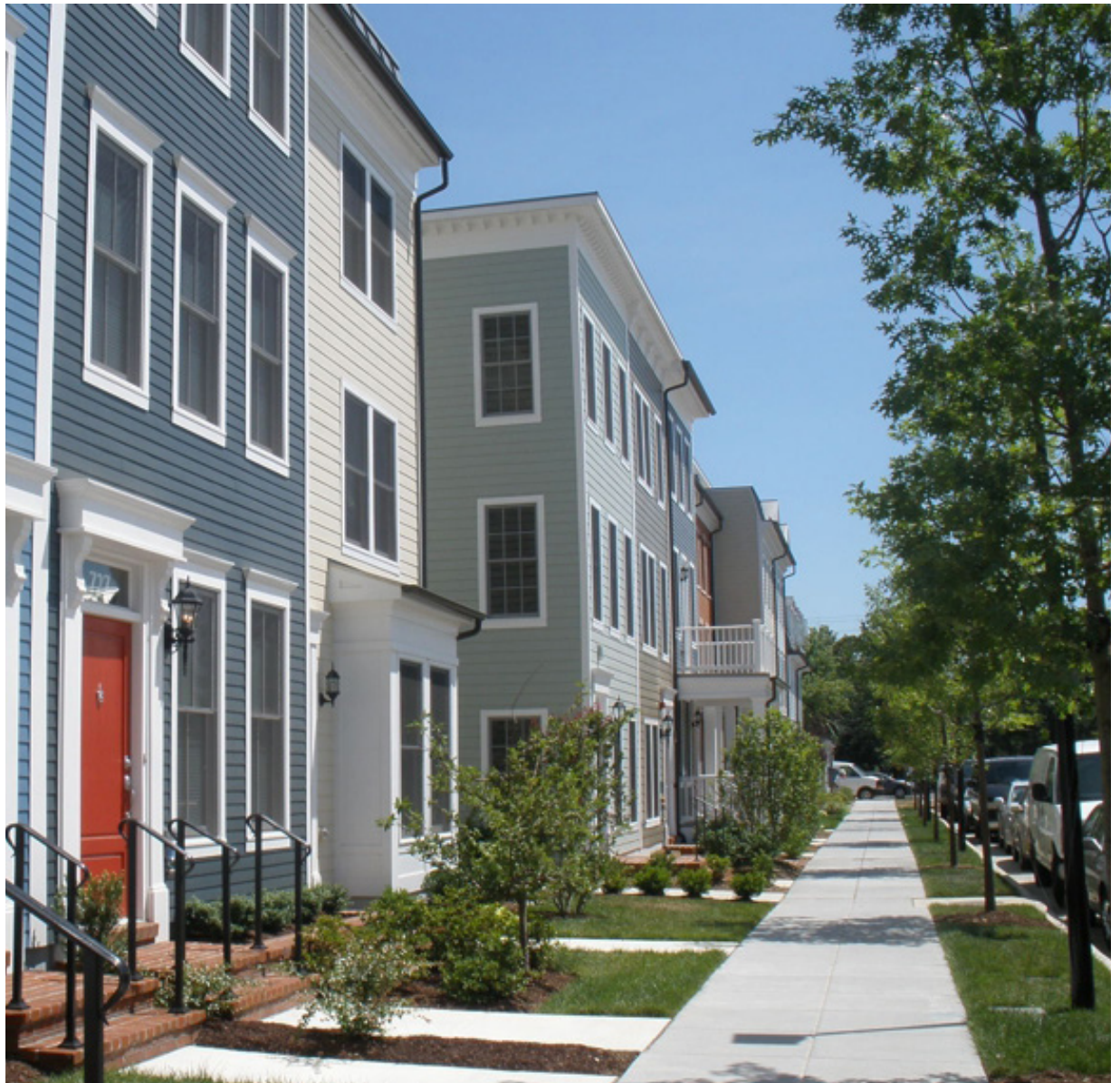
A residential street lined with townhomes, planted Frontage Zone and Planting/Furnishing Zone with continuous street trees. Source: movingtonova.com
