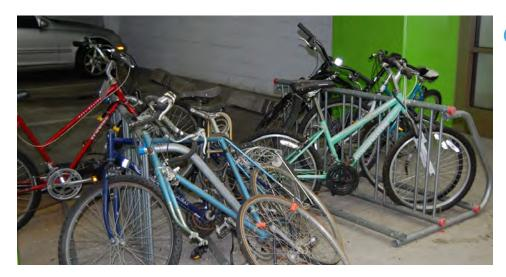
Schoolyard racks (top) and wave racks (bottom) do not support a bicycle with two points of contact leading to inefficient, haphazard parking that can damage bicycles.
