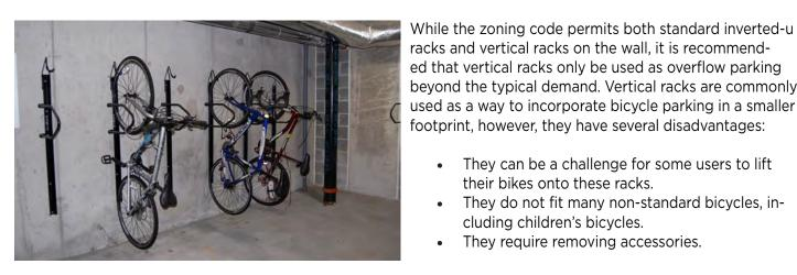
ed that vertical racks only be used as overflow parking beyond the typical demand. Vertical racks are commonly used as a way to incorporate bicycle parking in a smaller footprint, however, they have several disadvantages:
