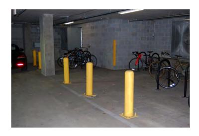
These bicycle racks are separated from motor vehicles by bollards.
