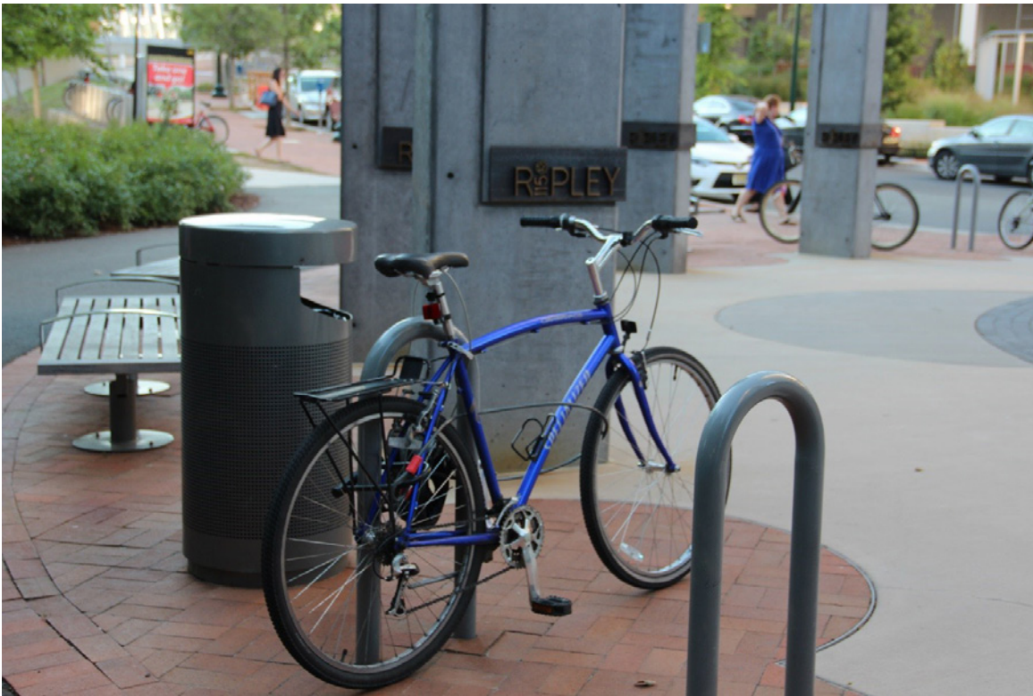
Short-term bicycle parking in downtown Silver Spring. The inverted U-rack shown here is the preferred short-term parking facility because it provides two points of contact for securing a bicycle; on the frame and on the wheel.
