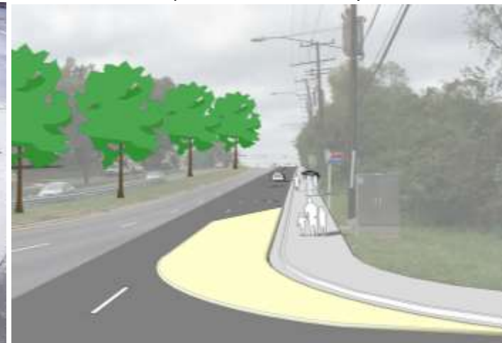
Modify existing right-turn lanes with engineering solutions such as curb extensions (Right Image Courtesy of Kittelson & Associates, Inc.)
