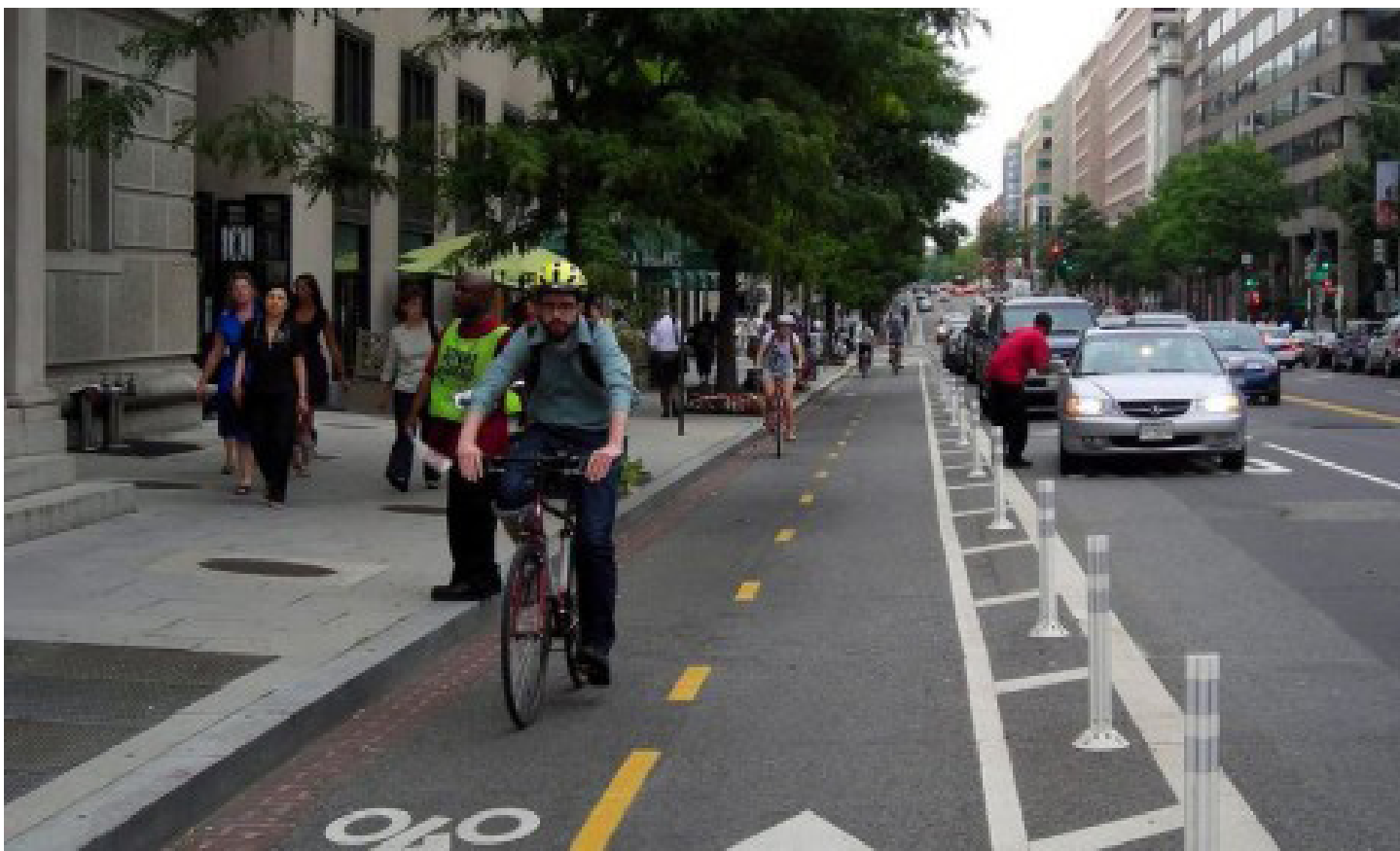
Paint and flexible delineator posts provide separation from traffic for these bike lanes in Washington, DC. Source: Toole Design Group
