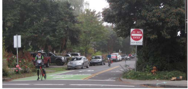
Bicycle box with lead-in bike lane
