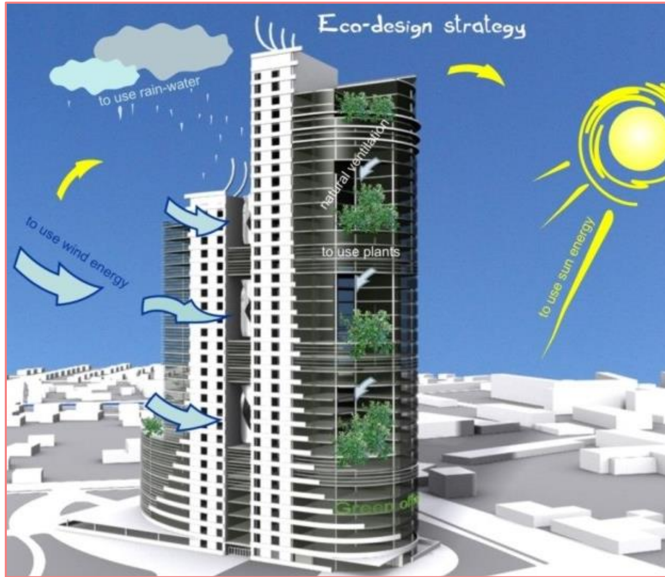
Example of building oriented to maximize natural heating and cooling
