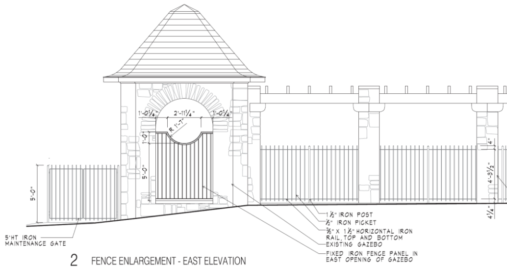
Figure 6: Detail image showing proposed fencing and change in grade.
