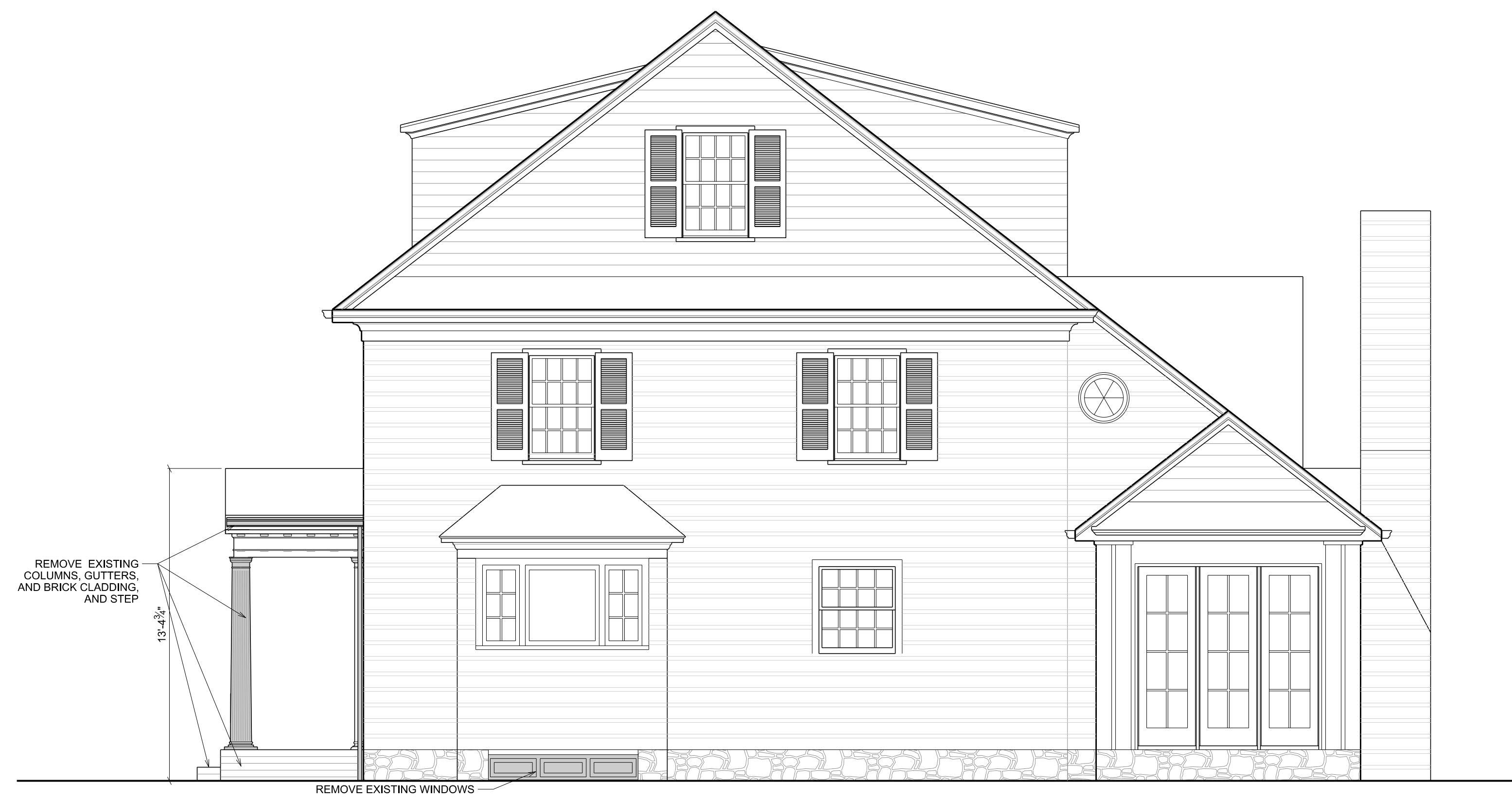
3 A003 EXISTING SOUTH ELEVATION SCALE: 1/4" = 1'-0" ■ DEMOLITION
