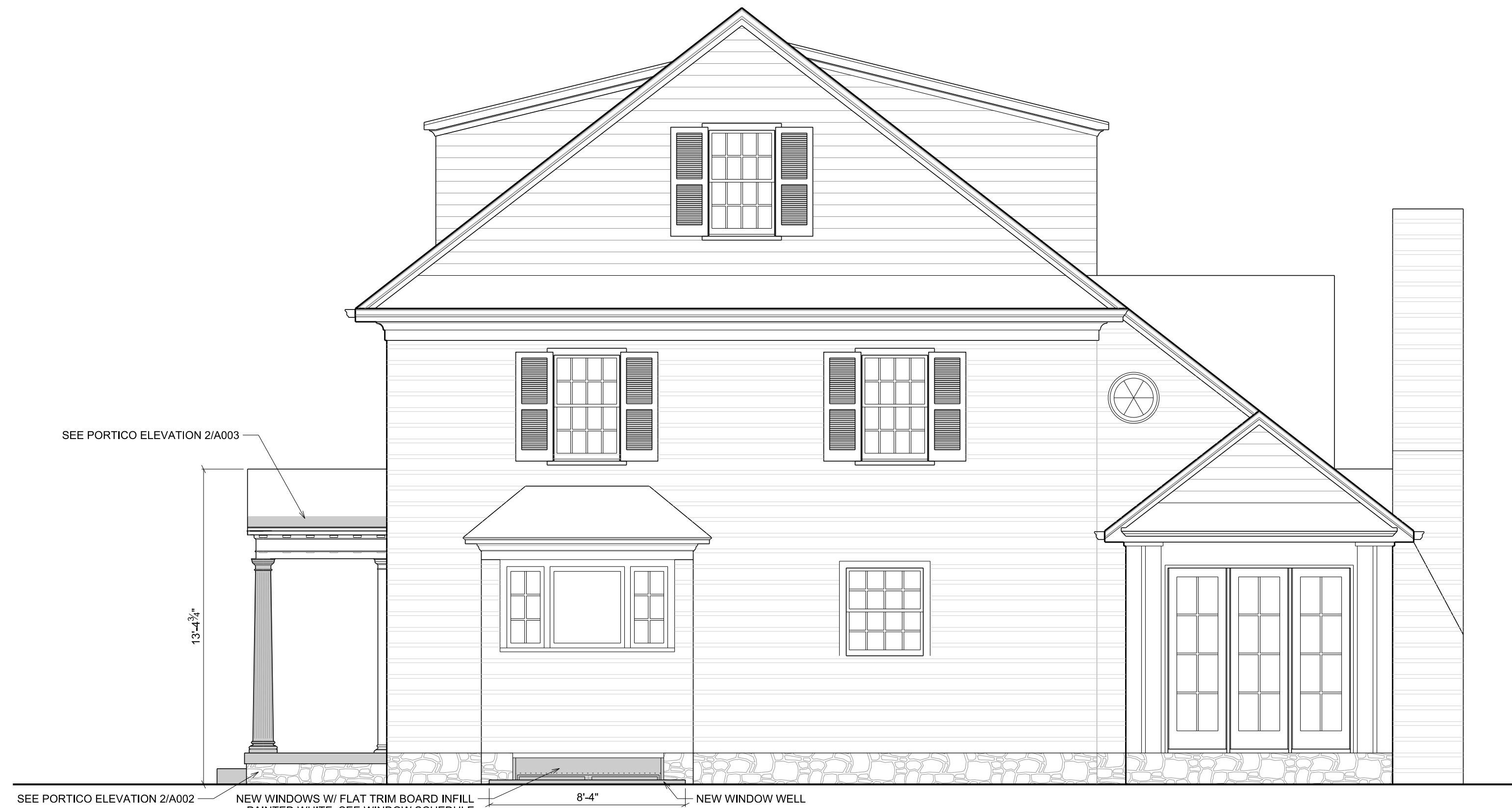
3 A003 PROPOSED SOUTH ELEVATION SCALE: 1/4" = 1'-0" ■ NEW CONSTRUCTION
