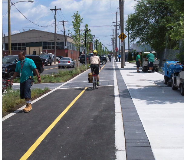
Example of a two-way separated bike lane with a sidewalk (Photo credit: Bicycle Coalition of Greater Philadelphia)
