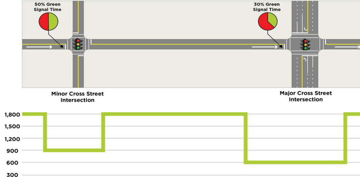
As shown in the above figure, the amount of green-time dedicated to cross streets is a main contributor to a corridor's overall capacity.
