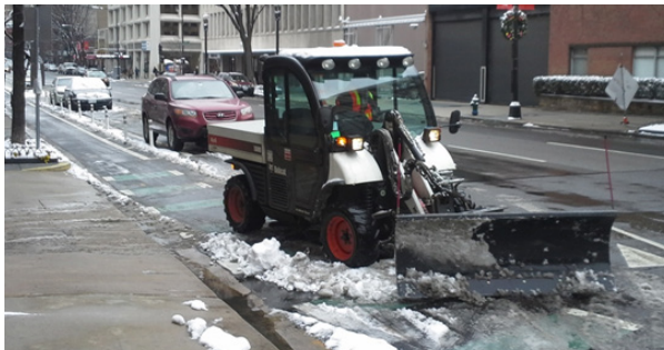
Plowing a separated bike lane with a smaller plow in Washington, D.C. (Photo credit: District Department of Transportation)
