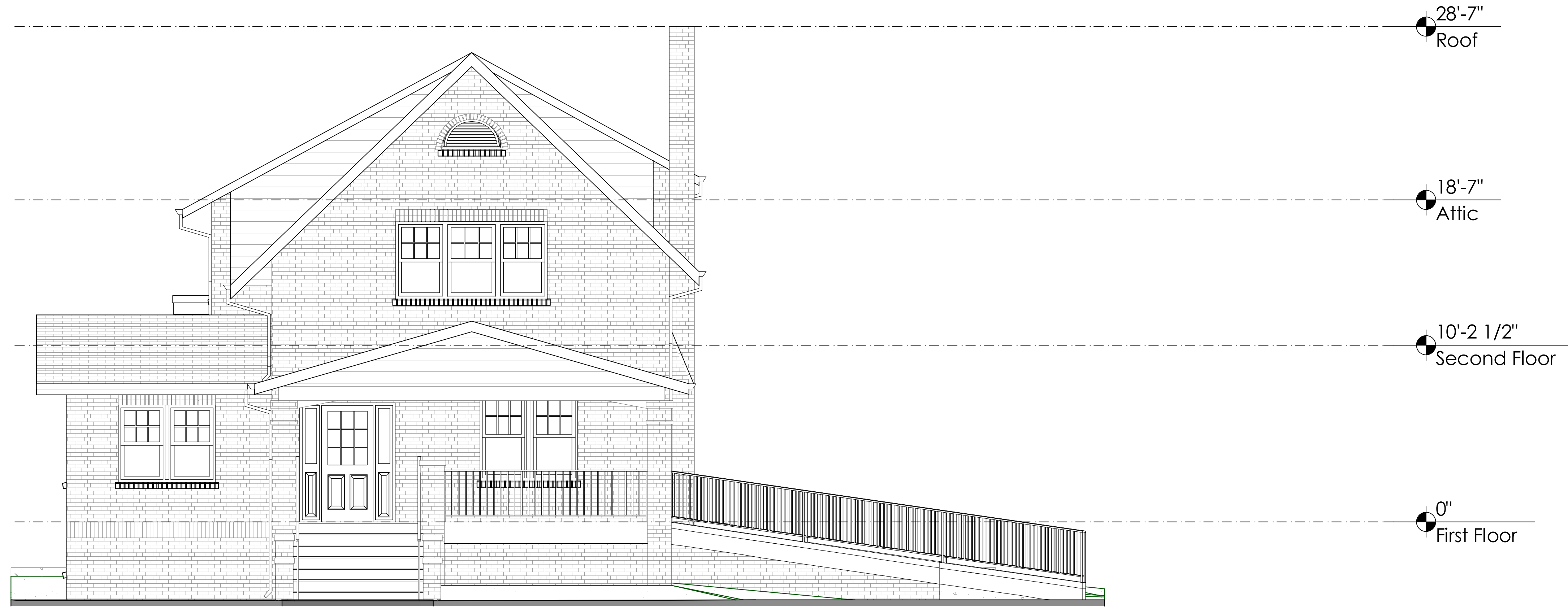
1 Front Elevation- Existing EX4 SCALE: 1/4" = 1'-0"
