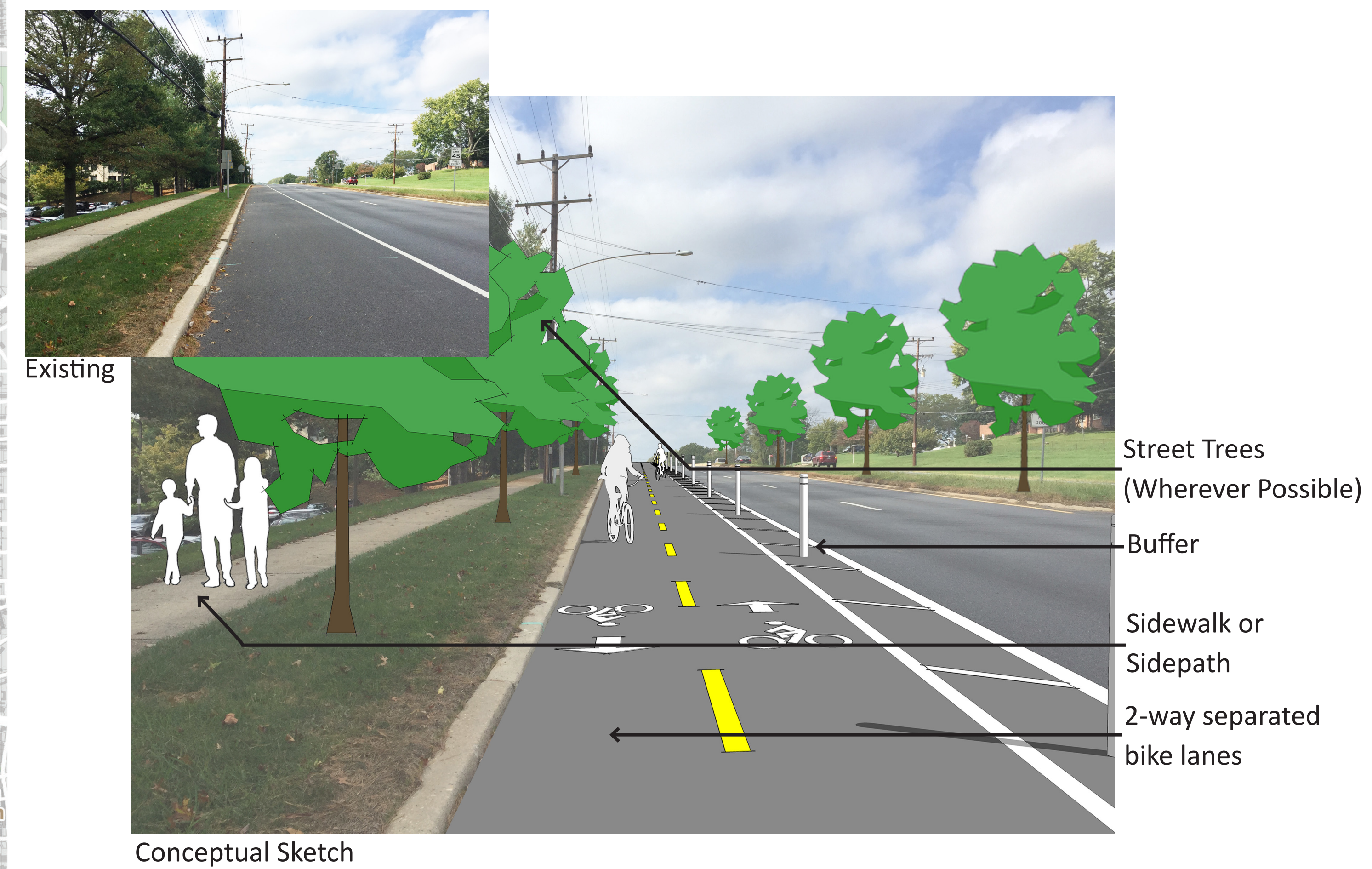
Example of a 2-way Separated Bike Lane
