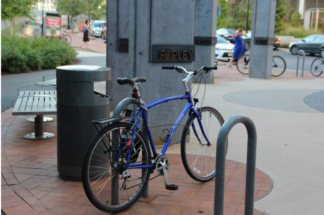
Short-Term Bicycle Parking in Downtown Silver Spring. The inverted U-rack shown here is the preferred short-term parking facility because it provides two points of contact for securing a bicycle; on the frame and on one of the wheels.
