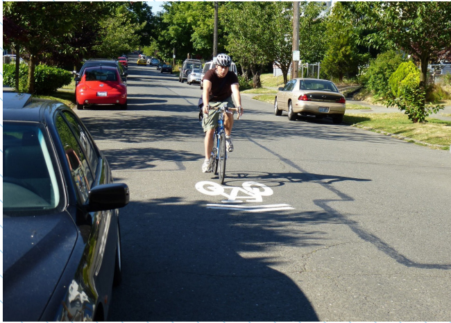
Sharrows indicate an appropriate path of travel to bicyclists and encourage drivers to move over to pass.
