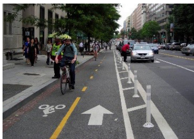
Example of Flexible Delineator Posts
