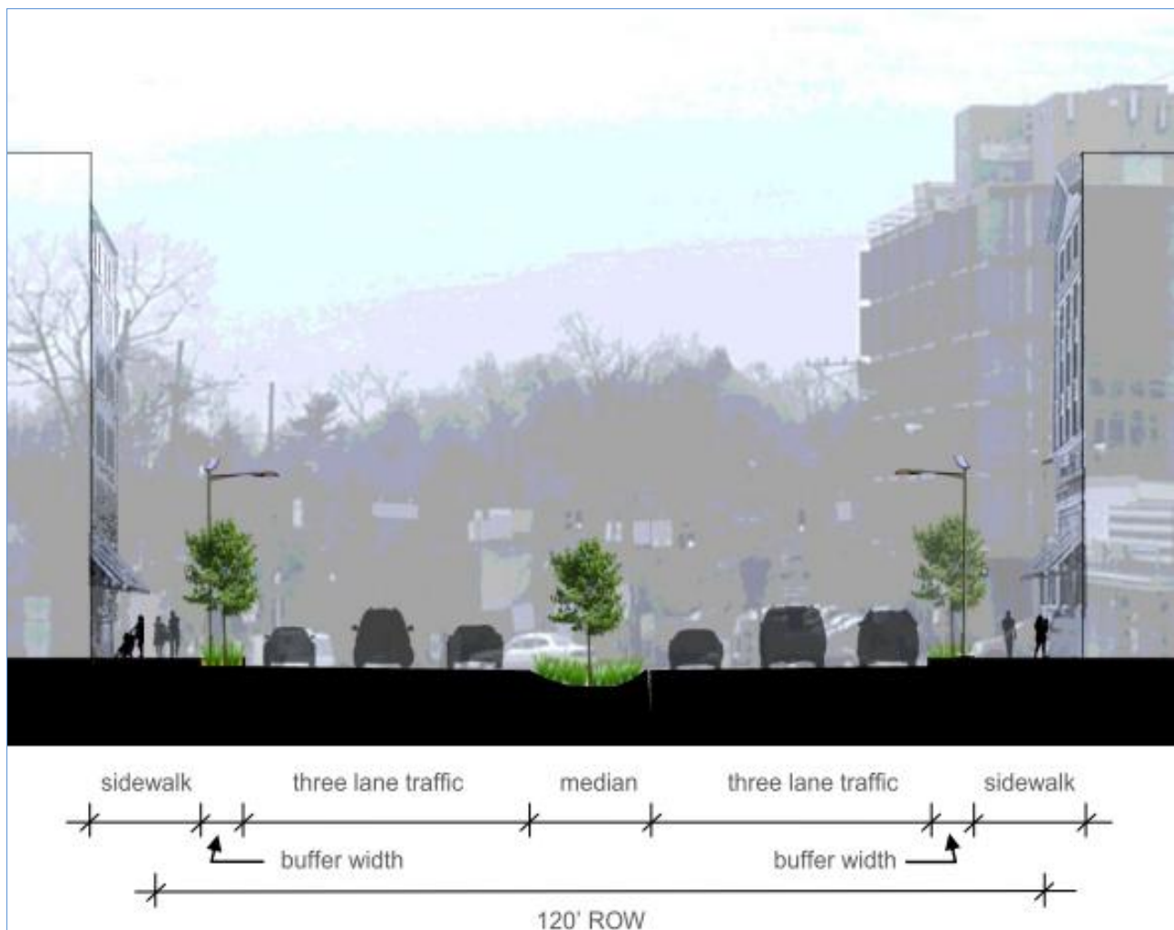
Figure B-4: Proposed cross section for Connecticut Avenue
