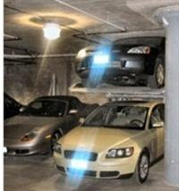
Car stackers allow two cars to park in one space, reducing the area needed for parking. They cost from \$7,000 to \$10,000 rather than the more than \$22,000 for constructing an underground space that would retail for over \$30,000.
