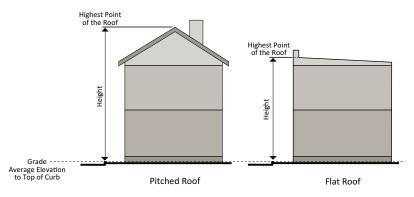
b. Grade is measured as the average elevation of the top of the curb adjacent to the front of the building. In a lot with more than one frontage, grade is measured as the average elevation of the curb along each frontage.
