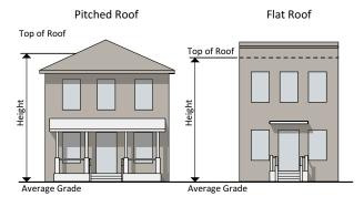
Average grade is calculated using the average of the highest and lowest elevation along pre-development or finished level of ground (whichever is more restrictive) along the front of the building parallel to the front setback line.
