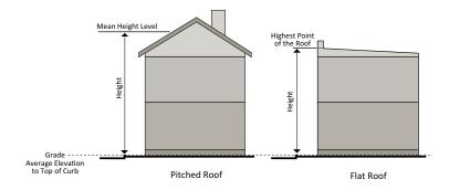
b. If a building is set back from the street line 35 feet or more, then the building height is measured from the average elevation of finished ground surface along the front of the building.
