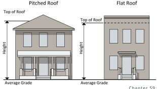
Chapter 59: Zoning Code Montgomery County, Maryland  Average grade is calculated using the average of the highest and lowest elevation along pre-development or finished level of ground (whichever is more restrictive), along the front of the building parallel to the front setback line.
