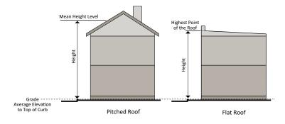
b. If a building is set back from the street line 35 feet or more, then the building height is measured from the average elevation of finished ground surface along the front of the building.
