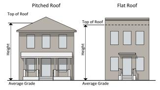
b. Average grade is calculated using the weighted average of point grades for each wall length along pre-development or finished level of ground (whichever is more restrictive), along the front of the building parallel to the front setback line. The weighted average of point grades for each wall length is calculated by multiplying each front facing wall section times the grade elevation adjacent to that section, summing all products, and dividing by the total length of the front wall.
