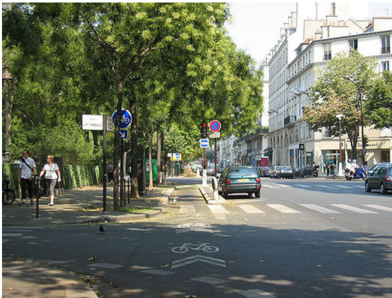
A multi-way boulevard is a system of parallel streets, within the same right-of-way, separated by a tree-line median. Local access lanes are incorporated to separate pedestrians, cyclists, and slower moving residential and commercial traffic from through traffic.
