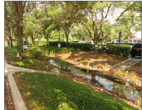
Orlando, FL: Landscaped islands in a parking lot provide an area for stormwater collection.
